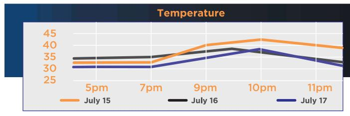
Based on a traditional approach using MDI data this transformer would have had to be replaced with a bigger transformer. But after reviewing the current and temperature data from the WMAC DTM it was obvious that although the transformer overloaded for periodsof time, was coping and there was no need to replace it with a bigger transformer.
