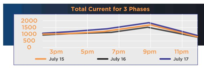
During the 9 to 10pm period, the 300KVA transformer was operating at between 130 and 150% of capacity, during this time there was no appreciable temperature increase measured on the oil tank.
